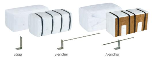
**SILCASTACK** and **SILCAFIX** systems are manufactured of special homogeneous, flexible fibre blankets with high resilience and classification temperatures of 1,260 – 1,600 °C. Able to be supplied in addition to gauze and tape modules are forms of execution with cords as well as also **combination modules**. At levels of compaction upwards of 200 kg/m³ the modules are manufactured as tape modules with plywood boards.
